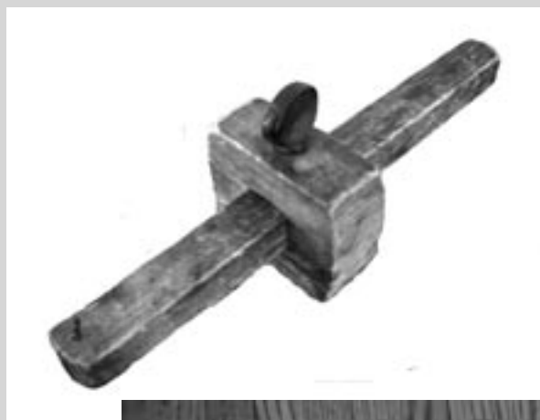
left: Marking gauge with tiny nail for measuring and marking wood.
