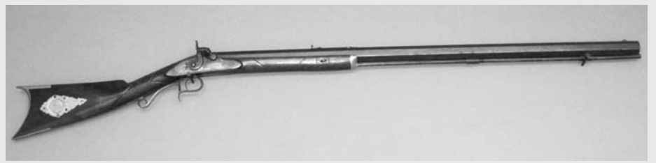
The Benjamin Schofield rifle is a black powder muzzle loader with a rifled 34" Heavy octagon barrel in .44 caliber.
